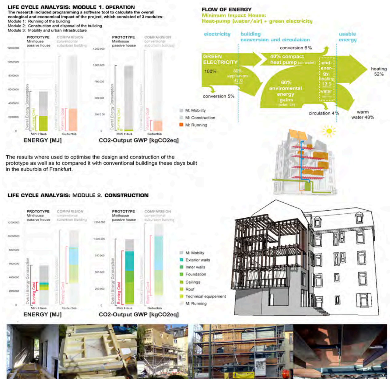
Fig. 5: Research project Minimum Impact House: Primary Energy Consumption in comparison to a conventional building construction
