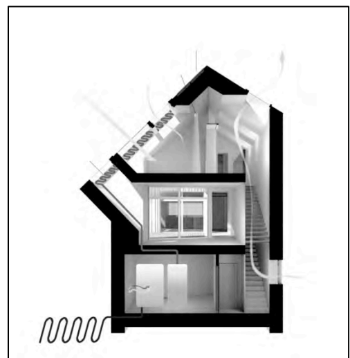
Fig. 6: Energy and ventilation concept of the Sunlight House
